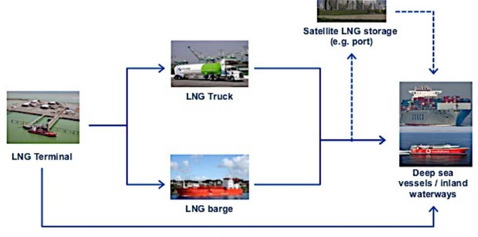
LNG bunkering options: Ship-to-Ship (STS), Truck-to-Ship (TTS), Terminal-to-Ship (TPS)
