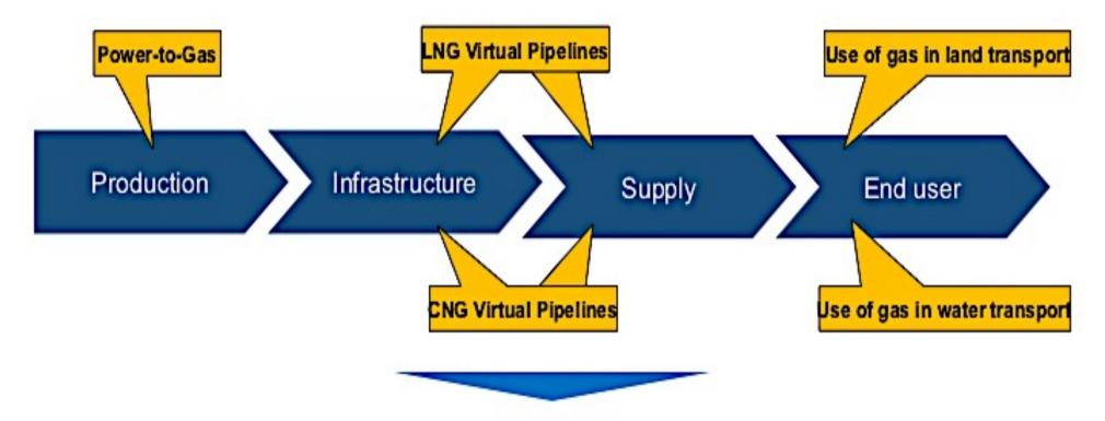
Virtual pipelines are closely related to the development of the use of gas in the transport sector, particularly in the case of LNG
