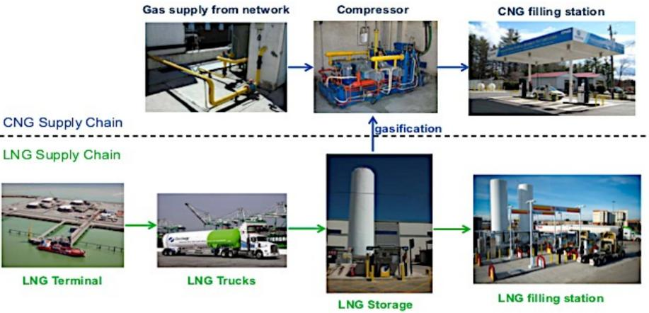
Virtual pipeline: the supply chain transporting natural gas to final consumers in the form of CNG or LNG, using road and
