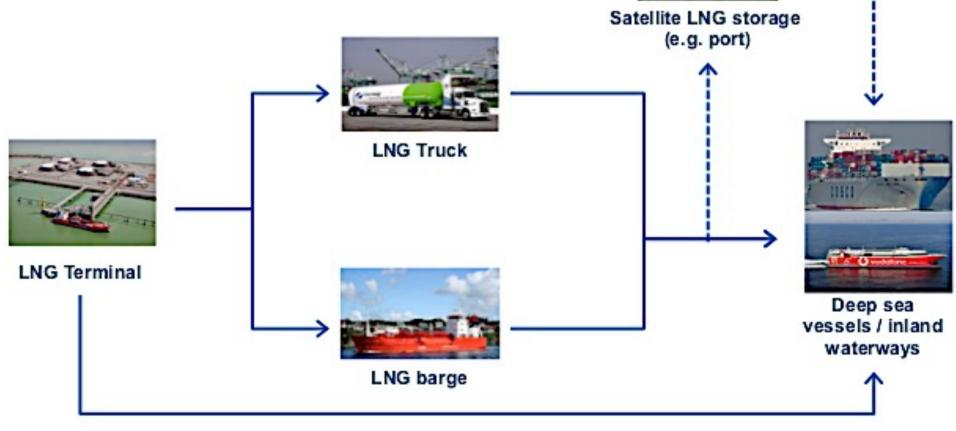
LNG bunkering options: Ship-to-Ship (STS), Truck-to-Ship (TTS), Terminal-to-Ship (TPS)
