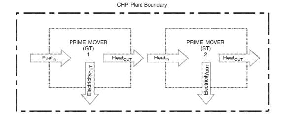
7. When the first prime mover is not producing electricity or mechanical energy, the boundary of the cogeneration unit is around the second prime mover. The fuel input for this second prime mover is the heat output of the first prime mover.
