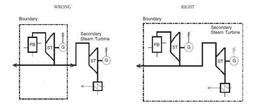
6. Where prime movers (i.e. engine or turbine) are connected in series (where the heat from one prime mover is converted to steam to supply a steam turbine), the prime movers cannot be considered separately, even if the steam turbine is located on a different site (see Figure 5).
